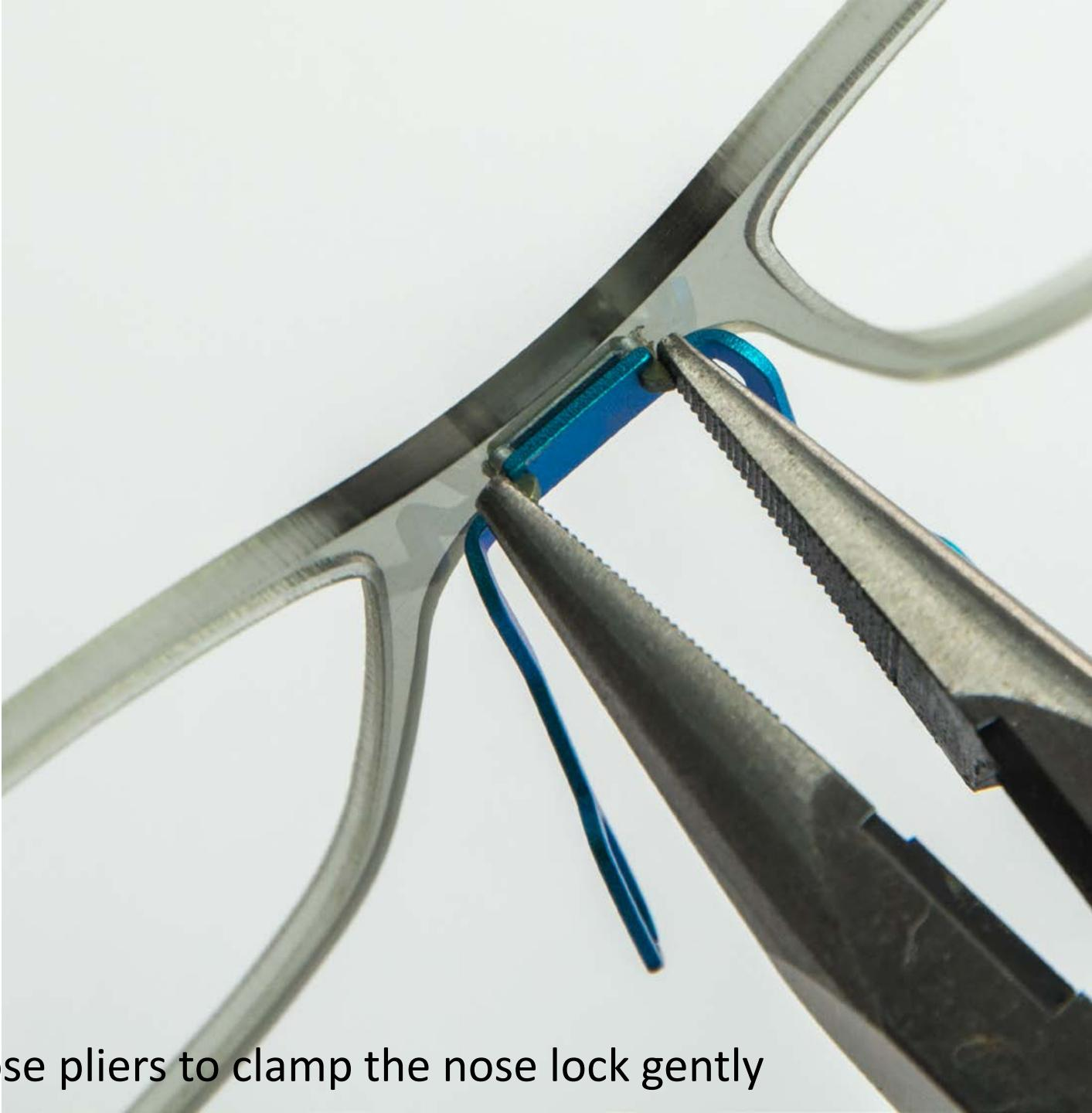
Take the needle-nose pliers to clamp the nose lock gently
