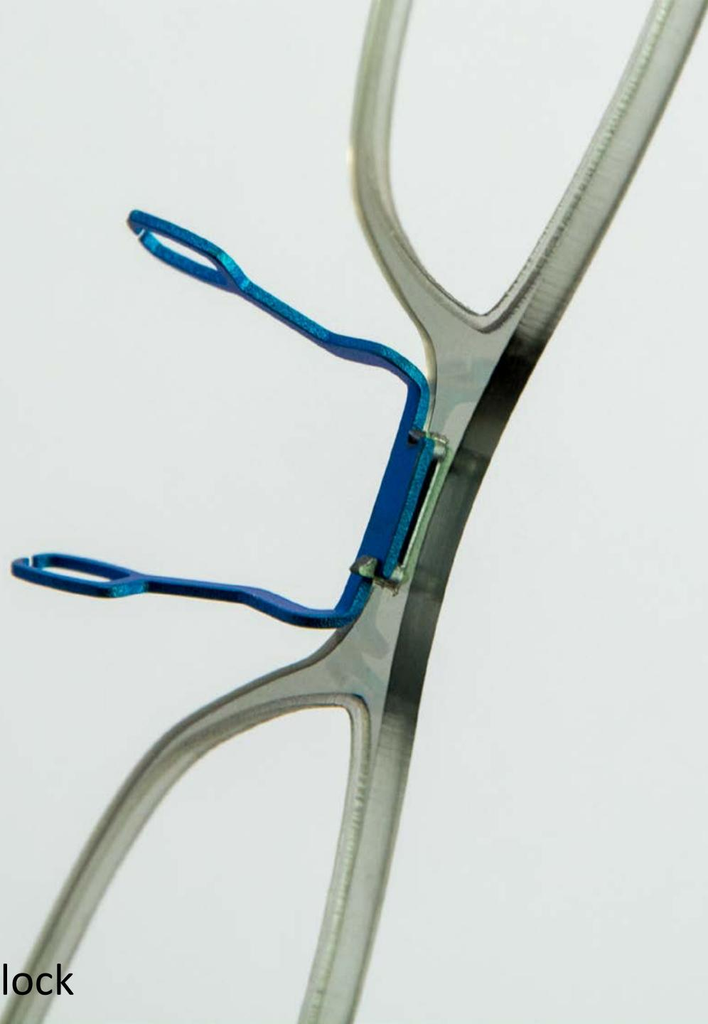
After cutting one pin of the nose lock
