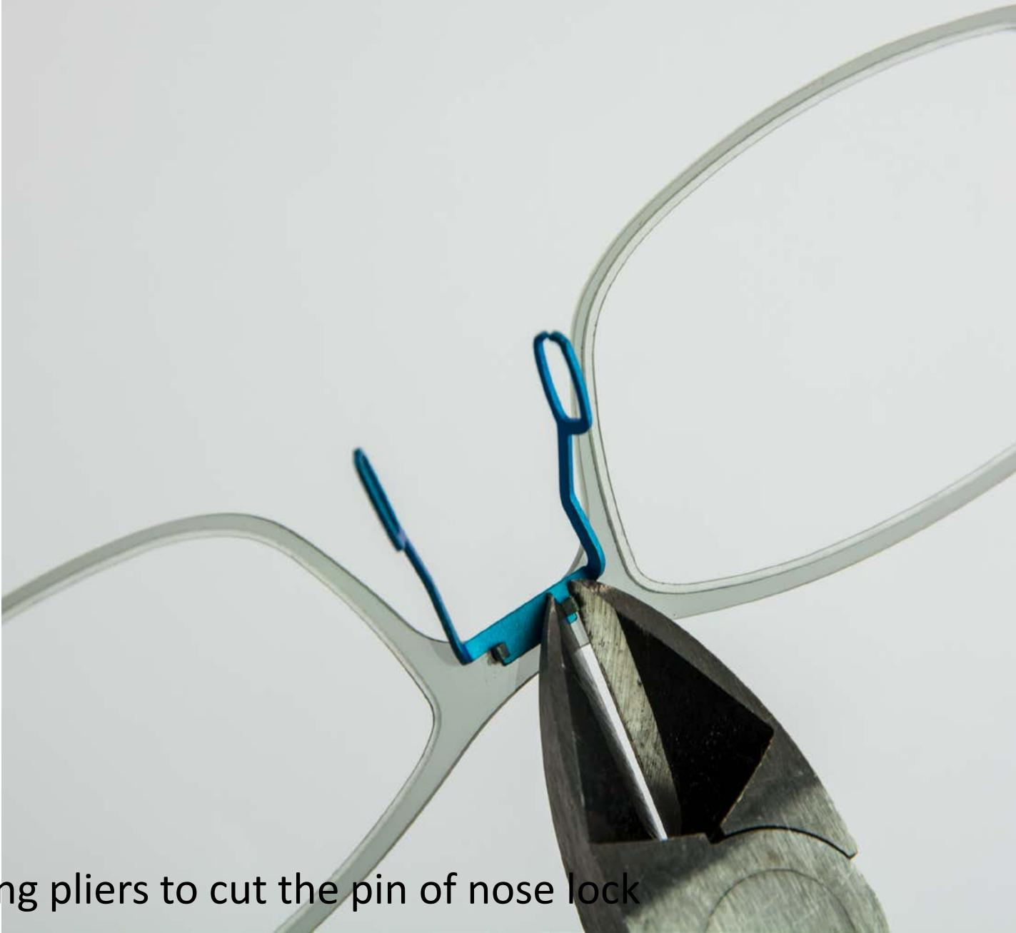
Take diagonal cutting pliers to cut the pin of nose lock
